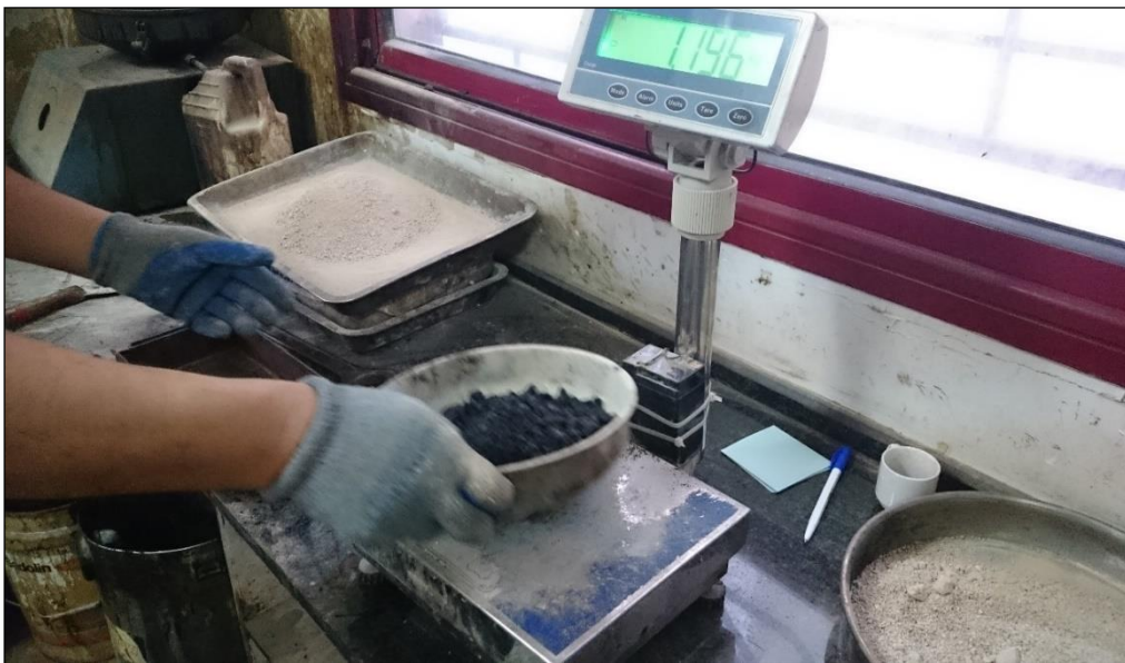
Figure E.4: preparing of marshal samples
