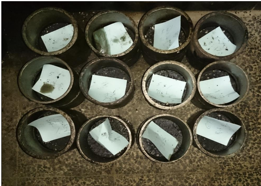
Figure E.2: Job mix marshal samples
