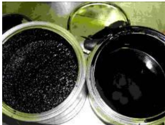
Figure (2.3): High viscosity (left) vs. terminal blend (right) rubberized binders
