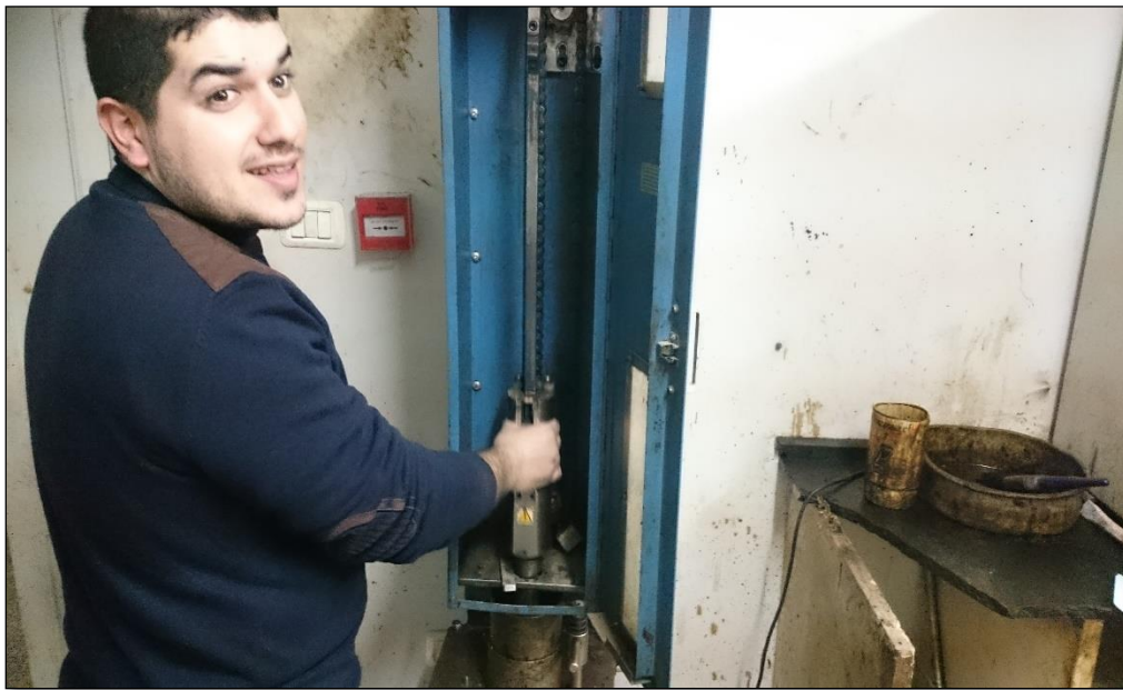
Figure E.7: Asphalt mix during compaction
