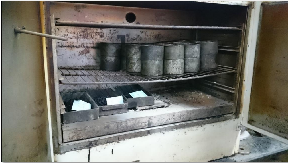
Figure E.3: Modified aAsphalt mixture samples in oven
